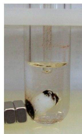
Figure 6. Retrieval of the magnetic \text{Fe}_3\text{O}_4 nanocrystals from a reaction mixture using an externally applied magnet.
